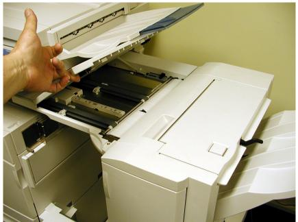
Figure 17 – The finisher's bridge misfeed-access area.
